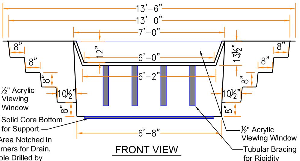
Drains can be Located in Either of the Four Corners
